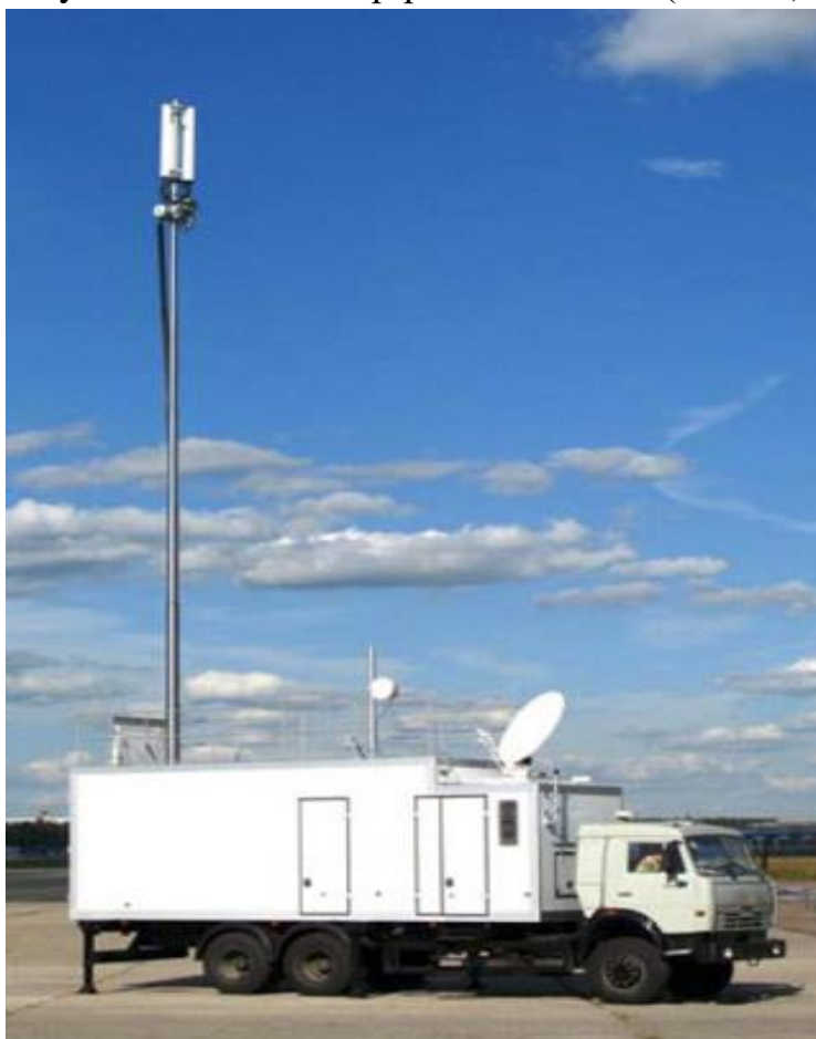
1-rasm. “Mobil” tayanch stantsiya “Kamaz” rusumli avtoyuk moshinasining ko‘rinishi.
